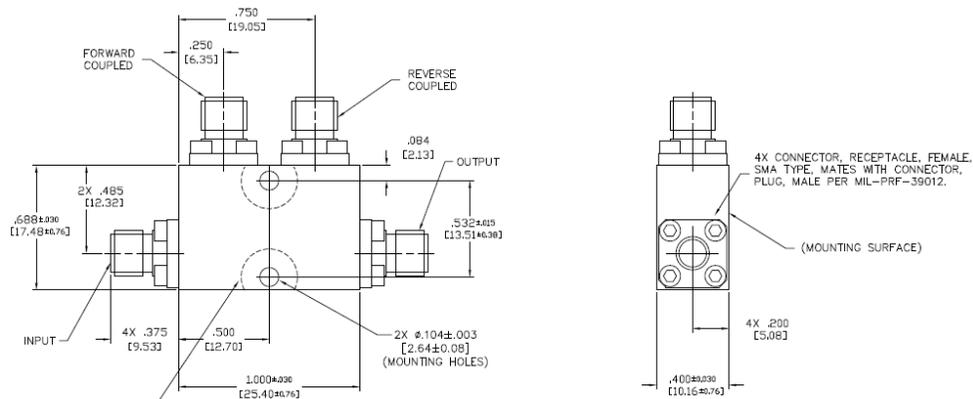
MOUNTING HOLE MUST BE FREE FROM PAINT .031 [7.87mm] AROUND HOLE. MASKING DIA. MUST BE CONCENTRIC TO WITHIN .020 [.51mm] OF MTG. HOLE.
