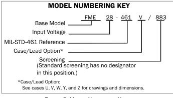
FIGURE 3: MODEL NUMBERING KEY
