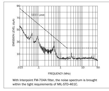
FIGURE 8: FILTERED DC-DC CONVERTER
