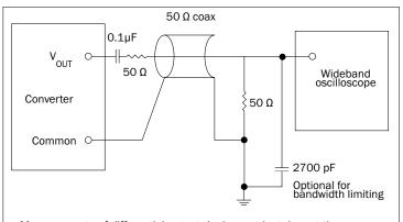
Measurements of differential output ripple must be taken at the converter's output pins to reduce the effects of radiated noise. Lead lengths must be kept to a minimum for the same reason. By adding parallel capacitance at the oscilloscope input, bandwidth can be reduced enough so that the ripple's fundamental frequency component can be viewed.
