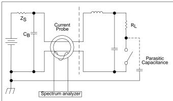
Common mode noise is caused by the collector or drain of the switching transistor. It forms a parasitic capacitance because of its closeness to the chassis. The noise can also be measured with a current probe.
