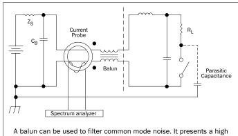
inductance to the common mode current and virtually none to the differential-mode current. Because the much smaller common mode noise current flows primarily through the bottom winding and through both windings in the same directions, the balun presents a high impedance to common mode noise currents.
