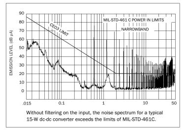
FIGURE 7: UNFILTERED DC-DC CONVERTER
