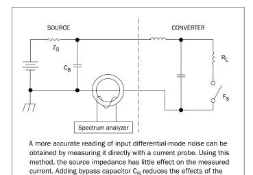
FIGURE 3: DIRECT INPUT DIFFERENTIAL MODE NOISE MEASUREMENT
