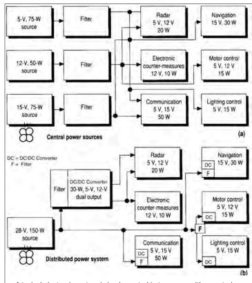
A typical electronic system is implemented in two ways: with a central power source (a), and with a distributed-power scheme (b). The distributed scheme illustrates the simplification and elimination of redundant wiring that can be achieved using that methodology.
