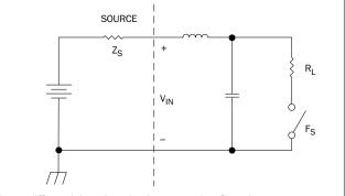
Input differential-mode noise is current that flows in a power system because of a voltage difference between the two input conductors. To control such noise, it must first be measured. Taking a voltage measurement across the converter's input terminals reveals the input ripple current multiplied by the equivalent source impedance.
