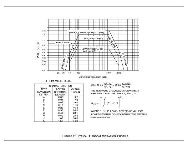
Interpoint does not screen for vibration except on a special order basis. We do however run qualification tests on new parts and, when vibration is included, we make sure that a resonance free mounting means is used. A resonance free means is achieved with an aluminum block, securely mounted to the shaker head, with cavities into which the power converters are inserted and then potted with wax. The vibration test may be run with or without power applied to the test samples.
