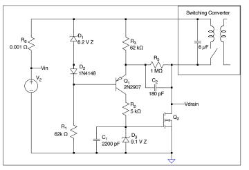
FIGURE 6: CONTROLLED RAMP VOLTAGE STARTING CIRCUIT
