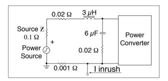
FIGURE 5: INPUT FILTER MODEL
