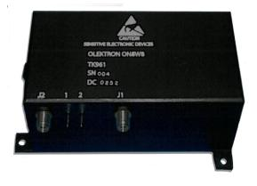
The unit incorporates a unique design that combines the frequency deviation of voltage controlled crystal oscillator with the stability of a temperature compensated crystal oscillator. Designed for use in a flightline environment, this oscillator combines unique features to meet
